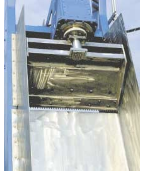
A scraper at the top of the stroke removes solids from the rake head.
