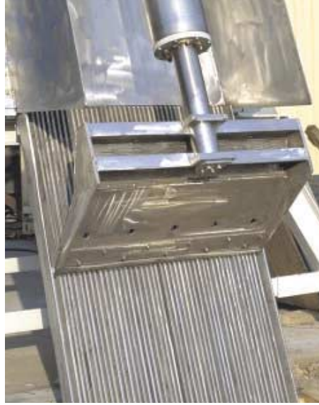
Solids captured on the screen are lifted by the rake.
