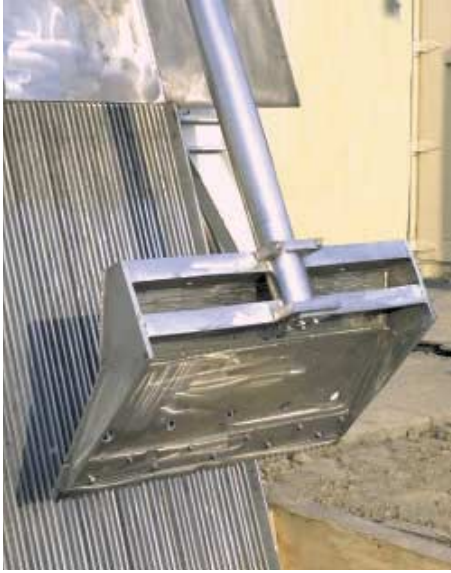
As the unit descends the boom pivots out.
